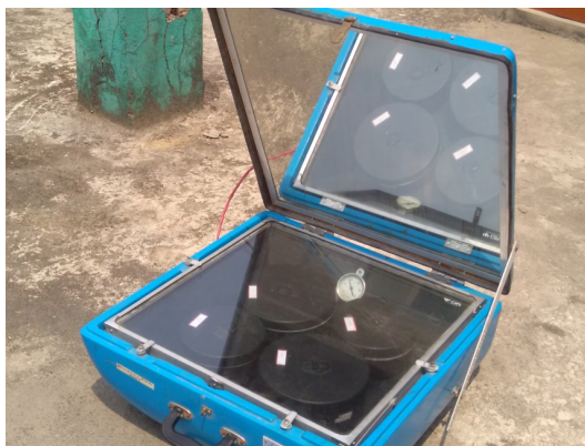
Fig.1.1. Box type solar cooker(a) Reflector, (b) Double glazing, (c) Aluminium container, (d) Temperature meter of the different parts in SDS
